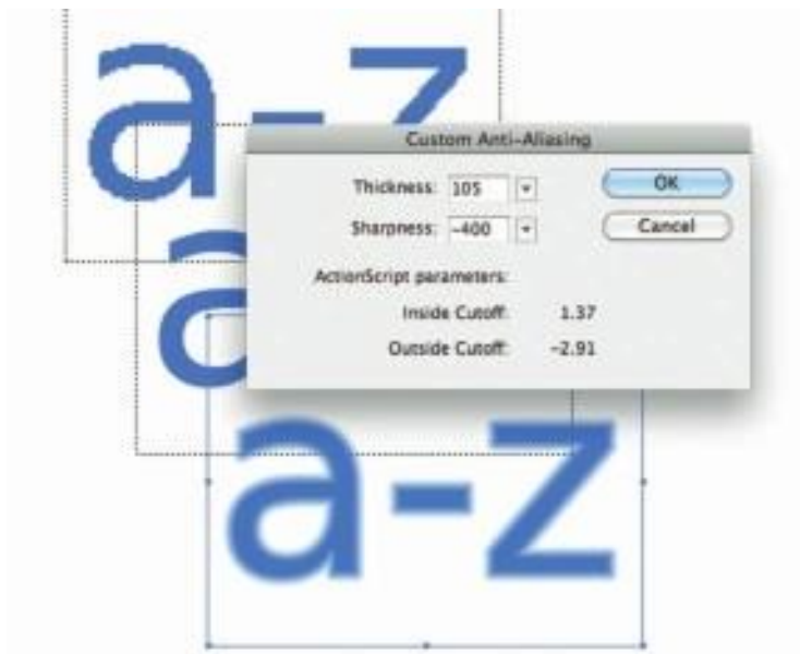
Figure 2-10 In some authoring programs, anti-aliasing can be fine-tuned.
